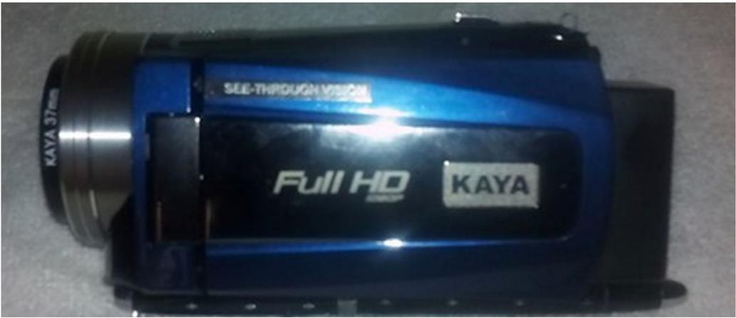
It comes with a pair of filters that when placed in front of the lenses they block all the visible light and just allow the passage of the near infrared rays giving with some materials the ability to see through them.
