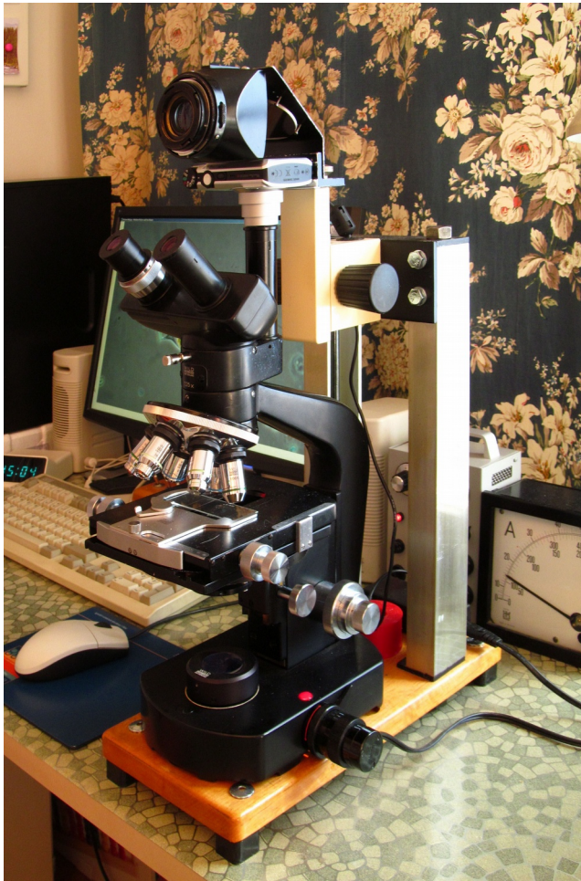
Picture 1 (left above): The M20 with Wild phototube and Canon camera A3200 with mirror and focusing magnifier (October 2015).
