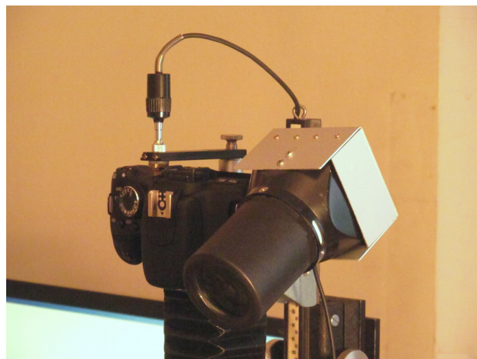
Picture 2 (right above): The M20 with alternative sliding stage (in front), Zeiss phototube, Exakta bellows and Canon camera EOS 600D with focusing magnifier and pneumatic release (September 2018).
