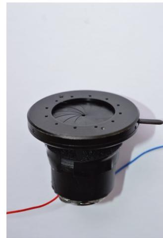
Fig.7. Mark II illuminator with diaphragm and magnet on base.
