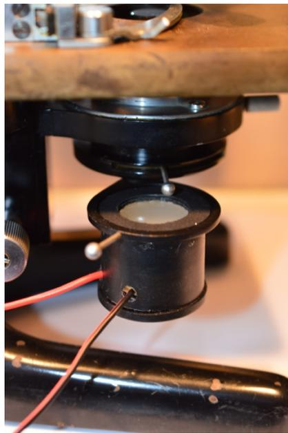
Figure 6. Card ring mount on Watson Service 2.
