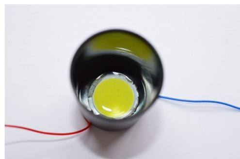
Figure 4a and b. LEDs mounted in film canisters with and without aluminium foil and diffuser disc mounted in canister lid before being re attached.
