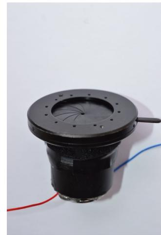
Fig.7. Mark II illuminator with diaphragm and magnet on base.
