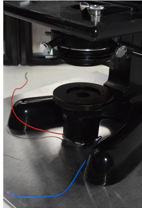
Figure 8. Beck 47 on steel sheet with magnetic Mark II illuminator being centred
