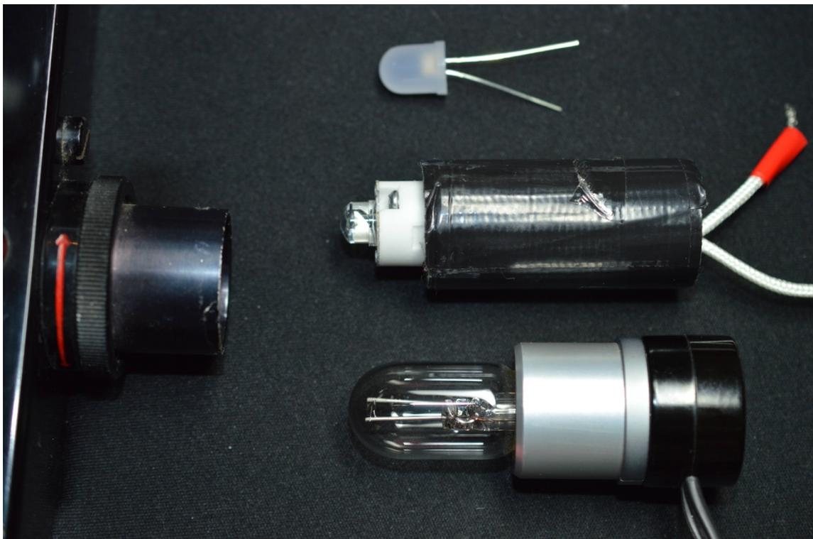
Fig 1. Wild M20 Replacement illuminator made out of broom handle cut to length with ceramic LED socket screwed in place, duct tape wrapped round to get snug fit. Straw hat LED mounted but can also use 10mm diffused LED
