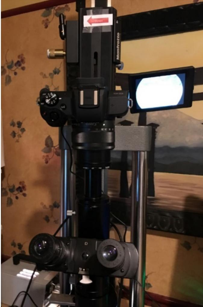
*Above: Afocal is just a camera suspended over a microscope. Not much to see here, folks . . . moving on.*
