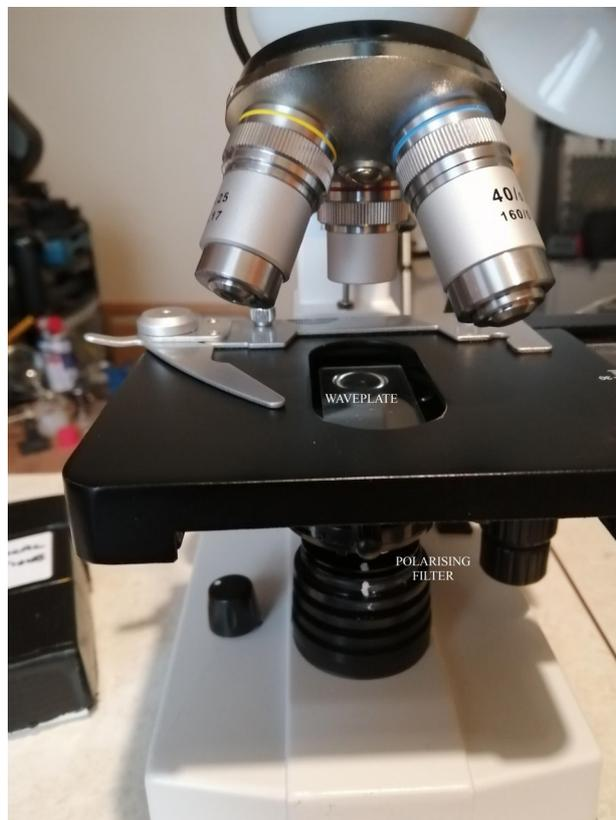
**Detail showing homemade polarising filter and waveplate in position on Apex Practitioner Microscope**
