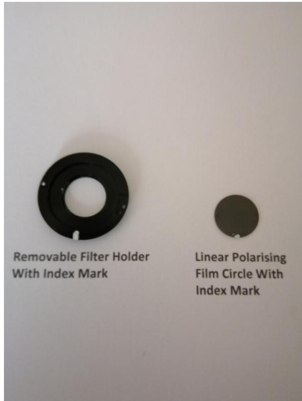
The polarising filter assembly was positioned immediately on top of the microscope sub-stage LED lighting unit (see picture above).
