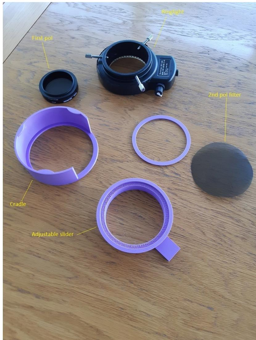
The idea being (not quite as expected as it turned out!) that light from the LED's would go down through the rotatable filter (2<sup>nd</sup> polariser) hit the specimen and bounce back up through the filter fitted into the head of the scope and thus view the specimen under polarised light.
