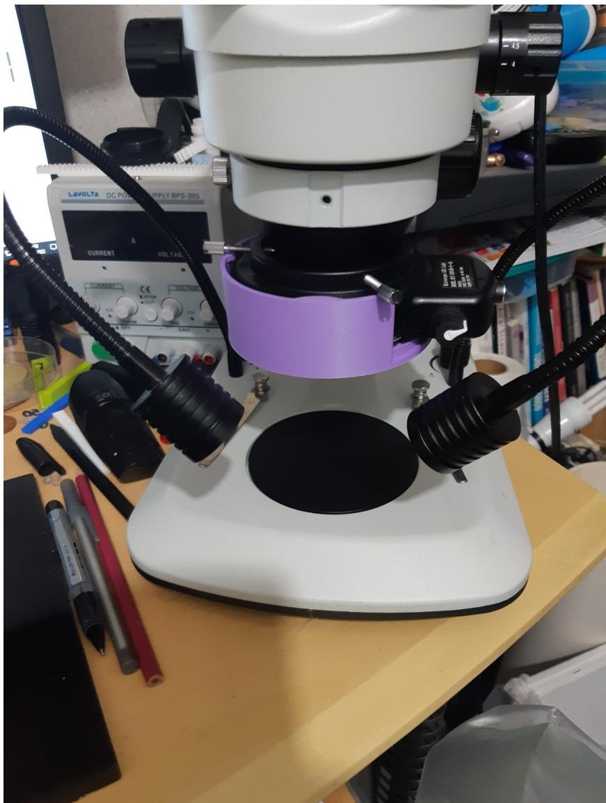
After some thinking I remembered I had a little used ringlight which I thought would give me the above light source which could somehow contain the initial polarising film. As others will know, to achieve cross polarisation requires two polar filters - one fixed the other rotatable to get extinction. And so after firing up the CAD software and then my trusty 3D printer this design came about!.
