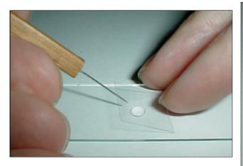
Gently lower the coverslip onto the diluted milk drop. Try not to make the drop too large, experiment a few times until there is little or no liquid creeping from the edges. Or mop up excess with a piece of tissue paper. (This is important to ensure you observe Brownian motion and not liquid movement caused by evaporation).
