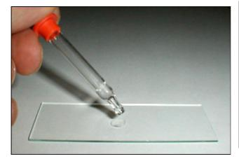
Place a small drop of water in the middle of the slide (use a dropper).
