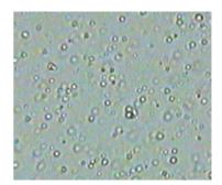
settled for a few minutes, the fat droplets should no longer be moving across the field but should be noticeably jiggling, but not in any specific direction. <u>This is Brownian motion</u>. Study the motion of the droplets on your own slide - how does the motion of the smaller droplets differ to that in the larger droplets, why?
