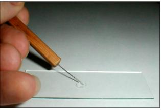
Dip the needle or wire in the milk, then dip and stir this wire in the water drop. (This ensures only very dilute milk is used.)
