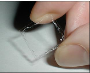
Optional: To make a slide that lasts longer, use a needle to lay a thin continuous line of Vaseline along the coverslip edges before lowering onto the slide. Also ensure the drop is quite small. Sealing the slide in this way minimises motion of the droplets caused by currents created by evaporation.
