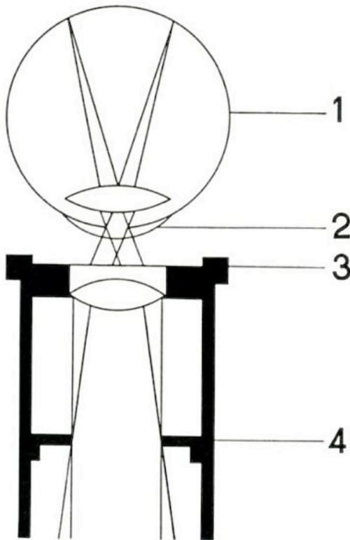
**Figure 6.** The line labeled “4” points to the ocular diaphragm. This is the point where to place the insert shown on figure 5.
