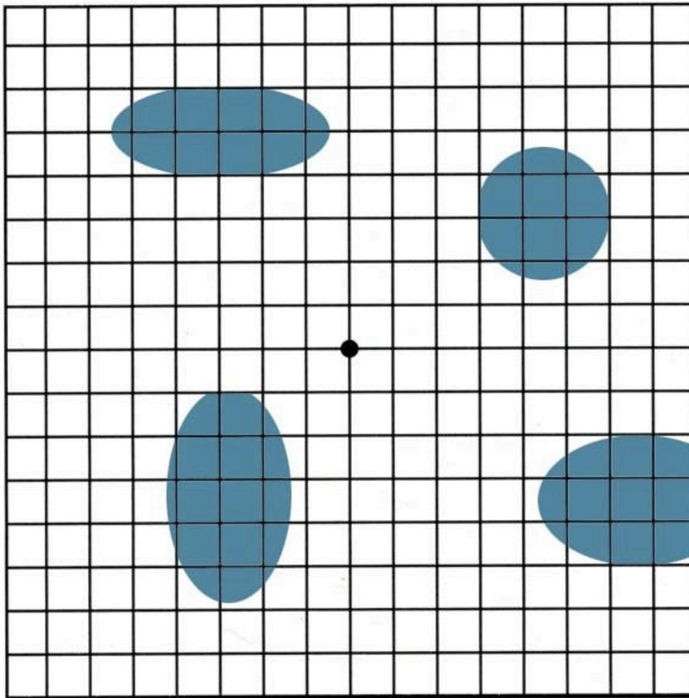
**Figure 2.** This diagram illustrates the application of the Delesse principle to a hypothetical random section. A grid is used as a testing probe and the number of hits on the whole field and on the particles is counted (further details in the text).
