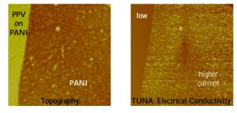
SPM can simultaneously record surface topography and a range of electrical properties including conductivity, surface potential and capacitance. In the
