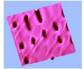
SPM can be used to identify a range of defects in CD and DVD maufactuiering processes. These can occur from defects in the original polycarbon ate moulds, errors in the stamping process and mastering mastering errors. SPM software can automatically calculate the pit depth, pitch and surface roughness and use pass/fail criteria to automatically identify defecvtive disks in a batch. In the image below, pit smearing ona CD is the cause of errors in audio playback.
