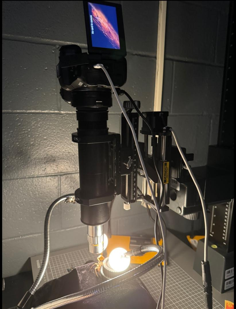
The image on the page shows the setup to capture the 10x image. The subject is set up below the Mitutoyo 10x optics lens system attached to the focus rail on the copy stand. The fiber optic lights are on each side lighting the subject. The other lenses were used for other magnifications.
