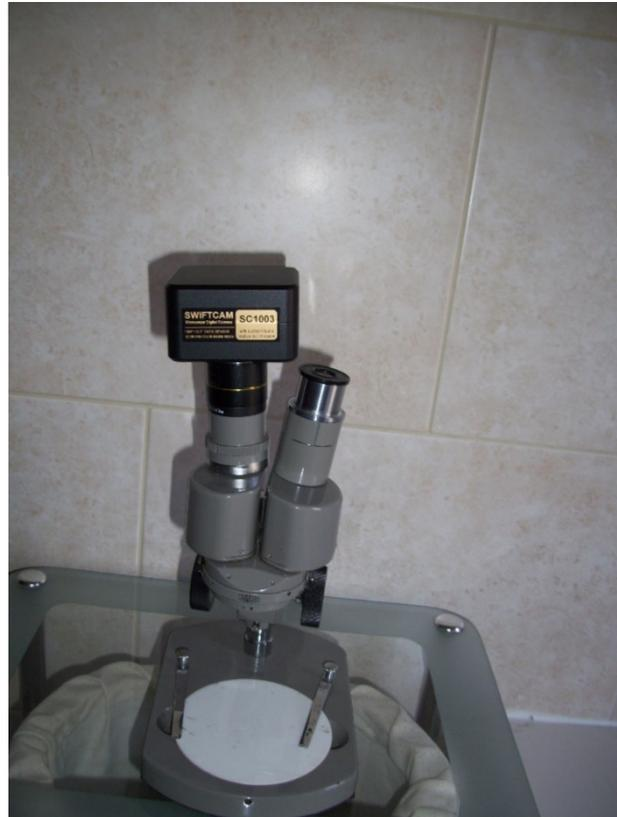
**Olympus VA-II stereomicroscope fitted with Swift SC1003 camera**
