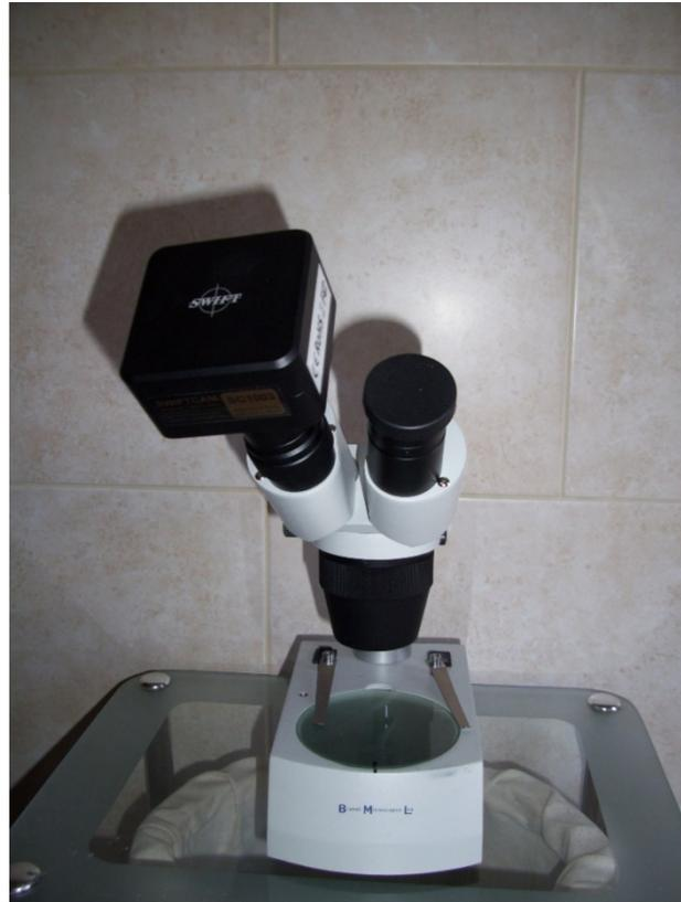
**Brunel Microscopes MX7T stereomicroscope fitted with Swift SC1003 camera**
