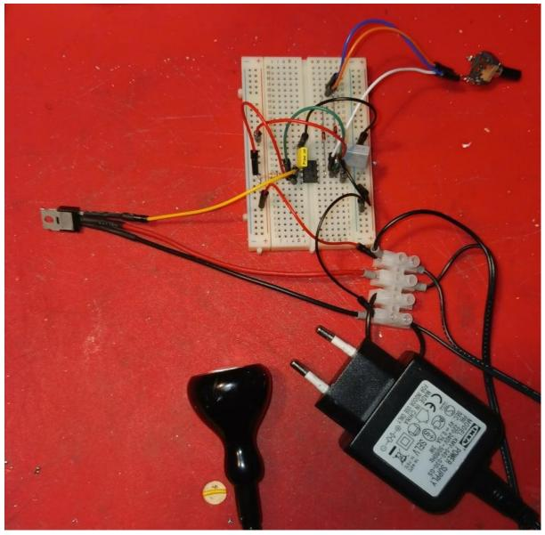
For pulse width modulation a 555 timer (controls duty cycle), switching transistor(s) and power source is needed.
