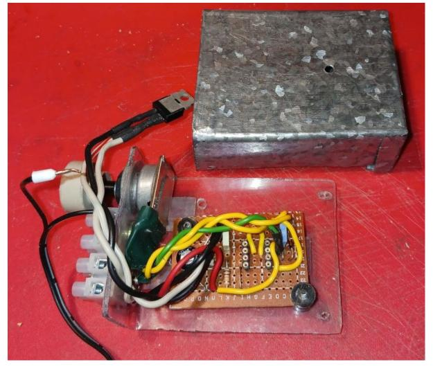
Layout chema is designed for breadboard and can easily be used with 'pre-drilled' soldering boards (you should not read this far, if you have capability to make your own PCB). With decent power, 47 uF capacitor can be omitted, it is for 555.
