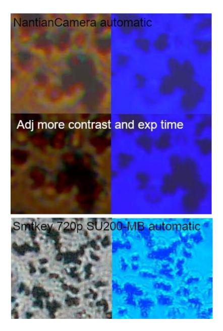
About the same area photographed with 3264x2448 (Nantian) and 1280x720 (Smtkey) sensors with white & blue light from Zeiss LgO (cell / sensor about 100mm above object plane).
