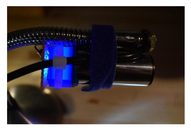
Here are plastic 14 mm stud + tape has been used to fit the board to 6X ramsden type eyepiece. Do not block airflow, but insulate components electrically.
