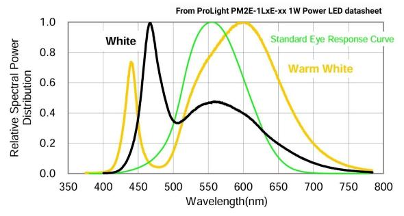
Traditional LED emits narrow one color spike. Big invention of Dr Nakamura was the invention of blue LED and adding a phosphorus layer which absorbs blue light and emits a wider spectrum. 'Blue' is about 450 nm. Jansjö (smooth) spectrum can be found: https://www.baertierchen.de/wb\_dez19.html
