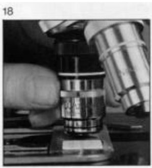
Iris diaphragm on immersion objective.
