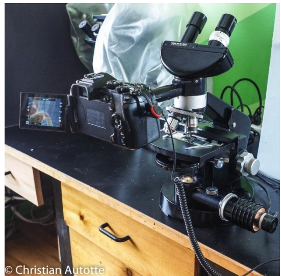
The Wild M20 with the photographic tube, which can swing independently from the binocular.
