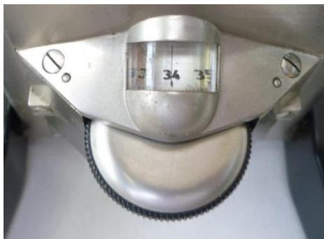
Coarse focus is with knobs either side just below the stage.
