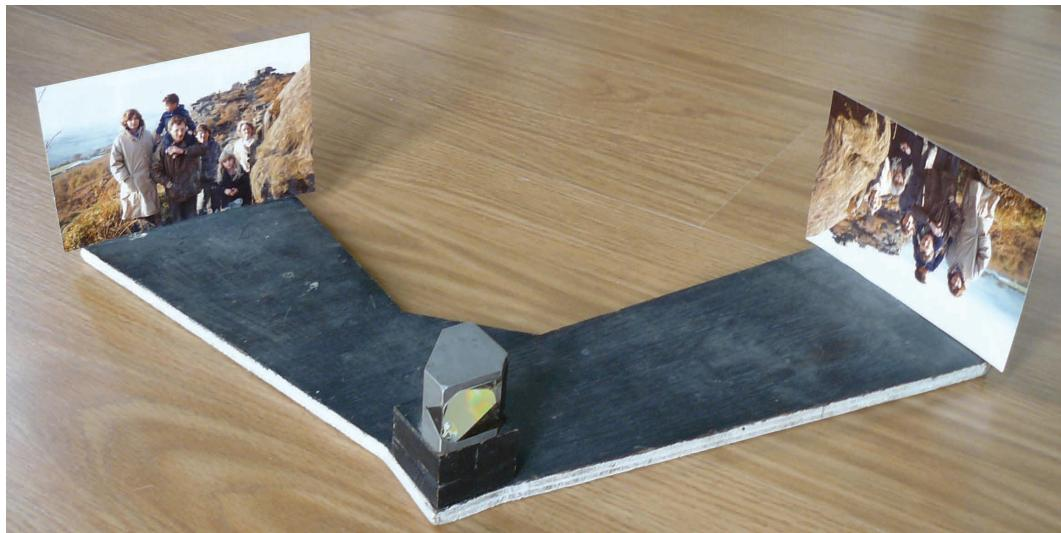
My plywood prototype made 44 years ago is shown in the photo. In that distant time computers were not available. Nowadays the ability to laterally invert the right hand image with one press of a button in a graphics program makes the roof prism itself redundant. This makes the construction of a stereo viewer with one simple 45 degree prism and a few bits of plywood simplicity itself. The photos can be held on the vertical back plates using a tiny spot of double sided tape.
