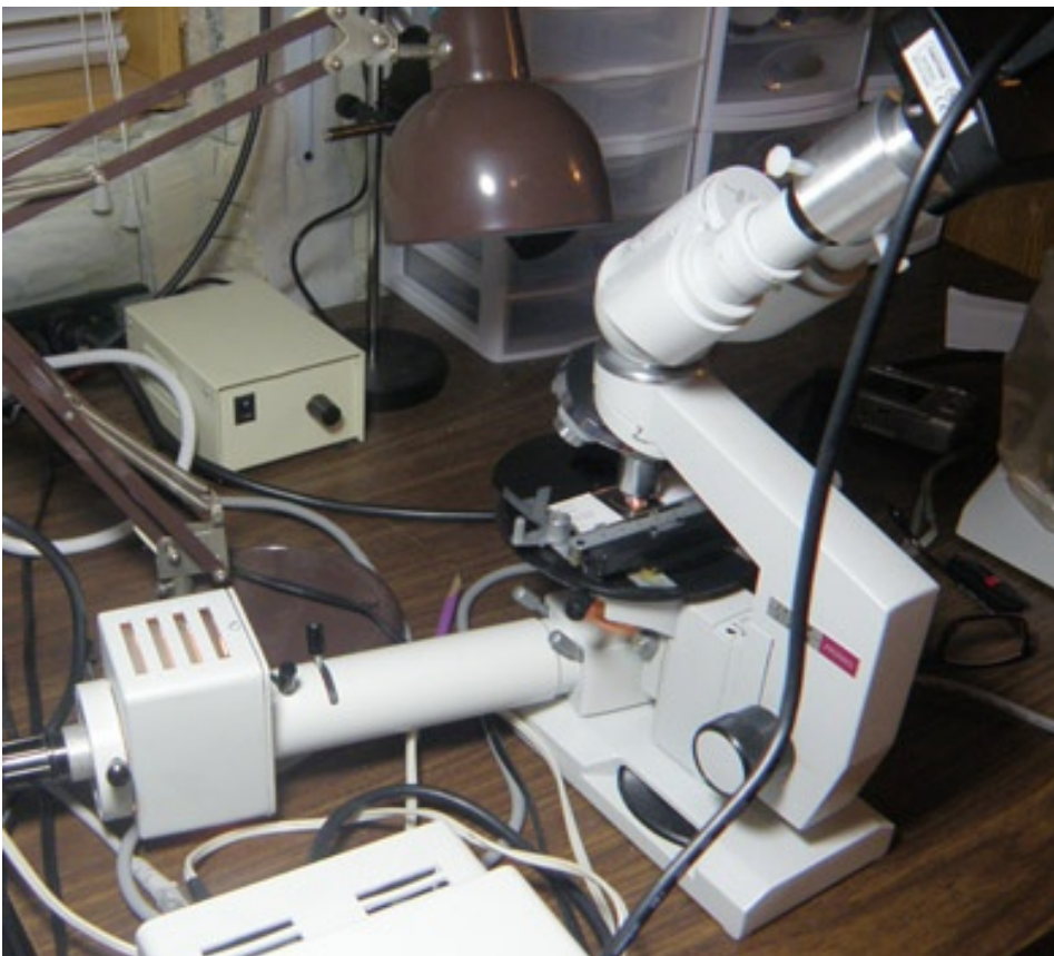
Lomo, Lomo illuminator, aplanatic condenser and apo objectives.
