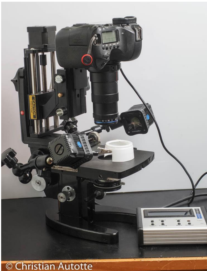
Two screws on the lens mounting collar neatly fit in the slot of the quick release plate, thus helping to keep everything perfectly vertical.
