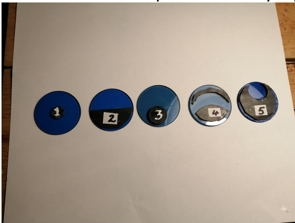
8mm diameter dark field stop and other variously shaped patch stops
