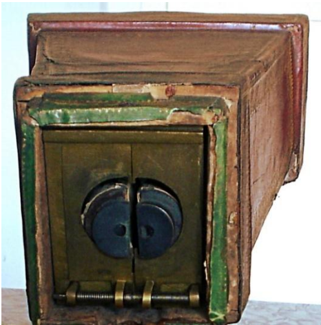
Figure 23 Left is the Anian microscope built before 1712 on Chérubin's design, right is its lower end with both objectives and its drive specified by Anian (Courtesy Deutsches Optisches Museum in Jena, Germany)
