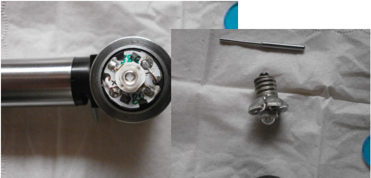
Photo 3. Light source, consisting of a 16 mm heatsink mounted on a 3.5 V bulb socket and secured with silicone heat glue.
