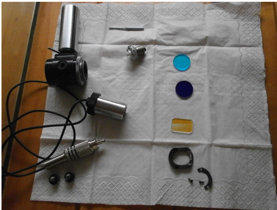
Photo 1. Parts of the illuminator transformed. The mirror dichroic is shown, approximately rectangular form. The filters SS-15 and SZS-21 (cut to 16 mm in diameter). The metal frame in which the mirror is mounted.
