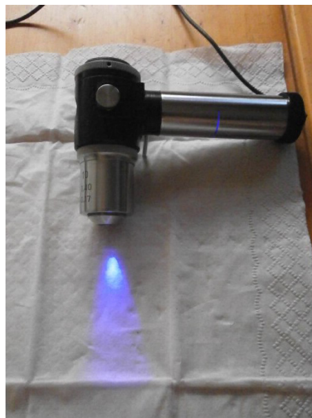
Photo 5, OI-1 Vertical illuminator with 10x luminescent lens and light source on.
