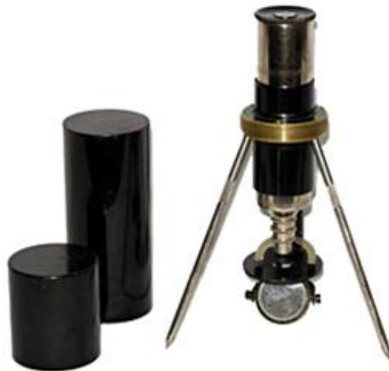
Figure 5. Spindler & Hoyer "Junior", Travel Microscope - Assembled for Use
