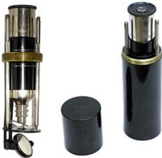
Figure 6. Spindler & Hoyer "Junior", Travel Microscope - Folded for Storage and in Case
