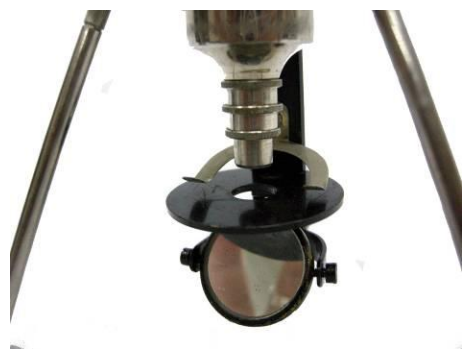
Figure 7. Spindler & Hoyer "Junior" stage, stage clips, and substage mirror
