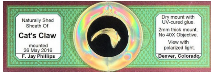
Figure 2. A dry mount using Lazer Bond UV-curing adhesive to attach slide components.
