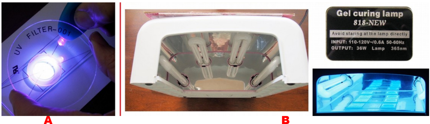
Figure 5. Curing UV adhesives. A. Curing one slide at a time with the LED built into the Lazer Bond glue pen. A UV filter from an old halogen desk lamp provides eye protection. B. Curing several slides at a time in a UV nail polish curing oven. A swing-down cardboard door on a tape hinge was added to block UV light while the oven is in use. Compact fluorescent bulbs emitting UV at 365 nm cure a tray of 8 slides in a minute.
