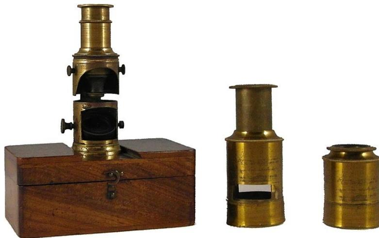
Figure 5. Bertrand "Furnace" and Pocket 'Live Box' Microscope Open and Closed
