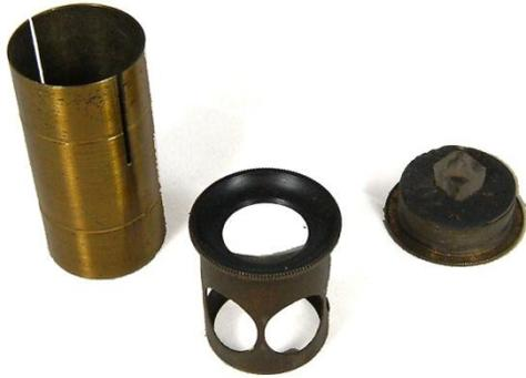
Figure 2. A Basic Cylindrical Microscope Disassembled to Show Removable Magnifying Glass
