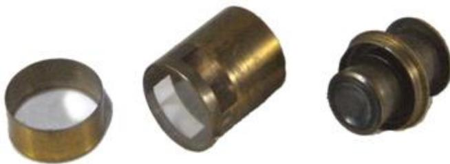
Figure 6. 'Live Box' Microscope Disassembled
