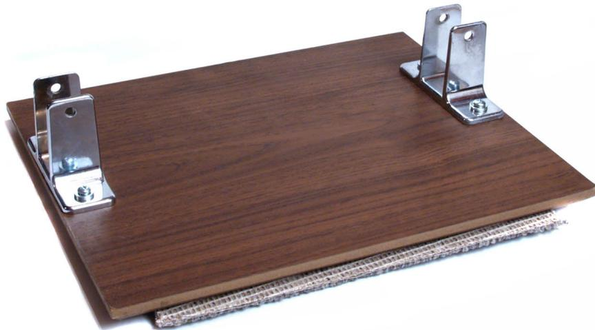
The chrome fixtures were from a box of hardware used to assemble restroom stalls that I purchased at a yard sale for two dollars. The next step was an upright plate drilled to accept U-bolts to mount the sander to the base plate.
