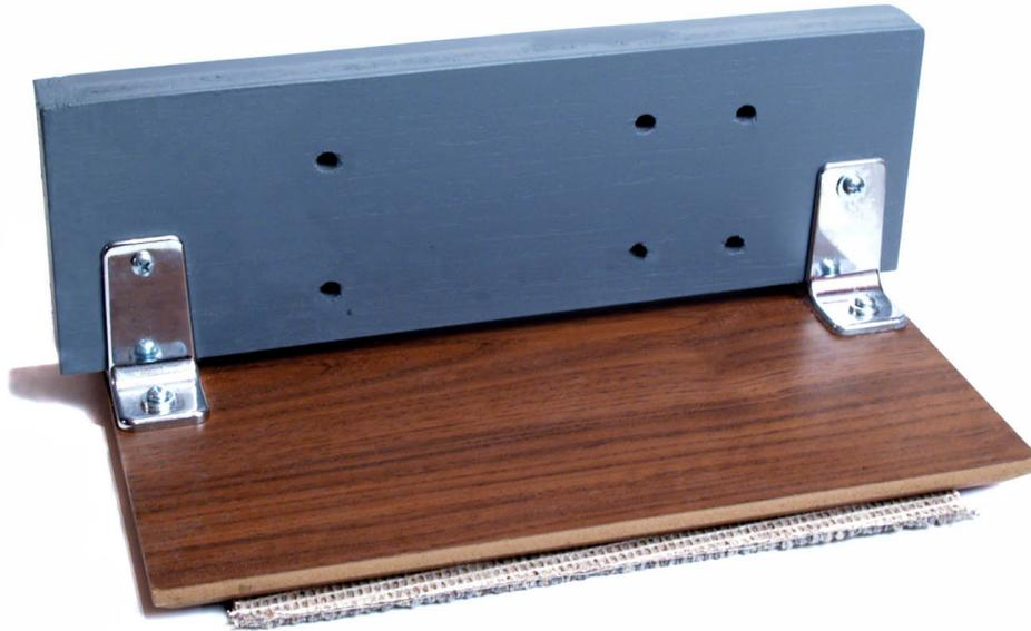
The last step was to mount the sander to the upright plate. The position on the upright plate is high enough to provide clearance to the on/off switch on the top (or, in this case, the bottom) of the sander
