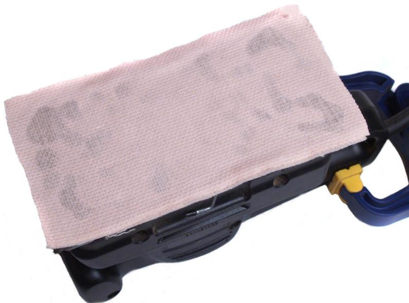
Once the glue on the fabric set, I glued the waterstone to the cloth using GOOP.
