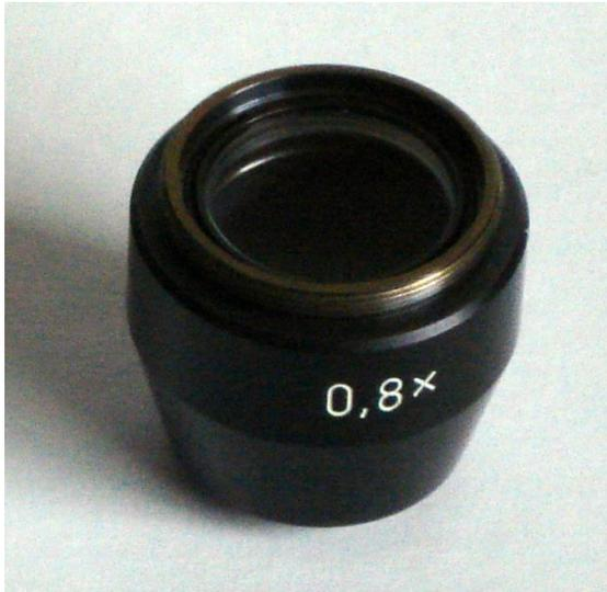
Users of Standard microscopes who wish to have the benefit of this large field can combine the small magnification changer 0.8x shown on page 3 or screw this 0.8x reducing system into their binocular tube which has, conveniently a 28x0.5 metric thread within the dovetail (compare the illustration of the binocular tube on page 2), or, as mentioned already, acquire the special Optovar with 0.8x as lowest factor. In each case a pair of Kpl 12.5x wide angle eyepieces completes the set-up.
