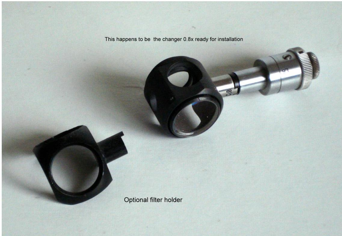
This is the magnification changer **0.8x** which I shall explain later on. The filter holder accepts standard 18mm dia filters. This could be a fluorescence barrier filter, an analyser or a neutral density filter. (I don't have a 1.6x changer nor a suitable photo, hence the 0.8x)
