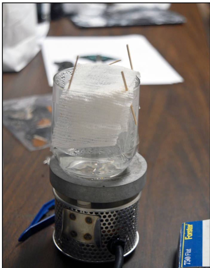
Fig 2.2: Toothpicks have been tacked between the upper gauze and the base gauze in this image to apply even and gently pressure to the subject. Once the subject cools it will remain in this position.
