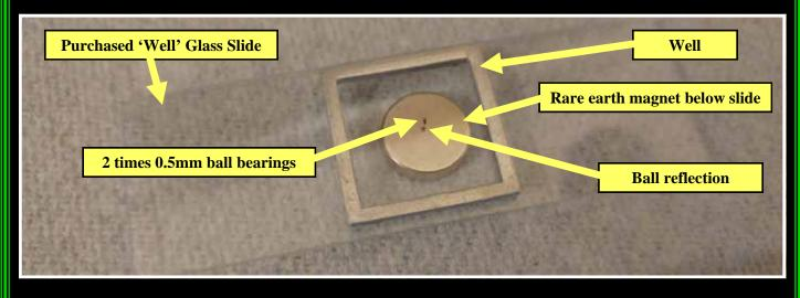
I used a very strong rare-earth magnet to hold the ball in the centre. I moved the ball/ balls to one side and put the ,merest hint of UV curing epoxy resin on the slide and moved the balls back onto the resin. I put the slide under a UV curing device for 6 minutes, a device used to harden a resin based polish in beauty parlours to decorate nails. You can see my set up below. One of the balls rolled off so I just used the one.
