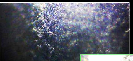
pictures were These two taken at 400x. They clearly show the ball is too rough and granular to reflect an image. The addition issue, is because of the narrow depth of field at increased magnification, the spherical
