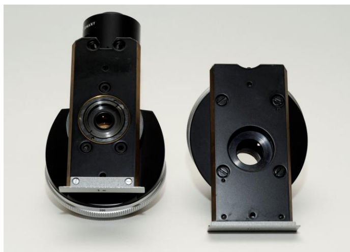
Figure 8 – Horizontal dovetail of the revolving nosepiece of the Ortholux II (left) and the Orthoplan (right).
