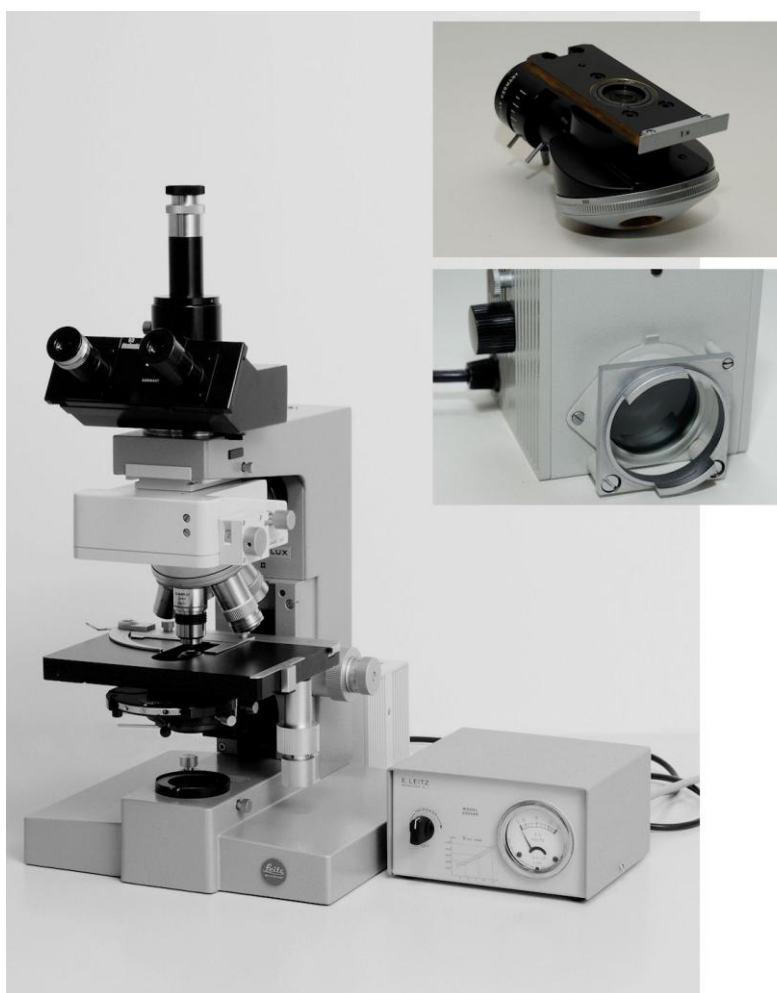
Figure 6 - Leitz Ortholux II with Ploemopak 2.2, FSA viewing head and Leitz 402a phase contrast condenser. The locking device of the Leitz Lamp Housing 50 and the episcopic nosepiece with a 1× tube lens are shown in separate insets.
