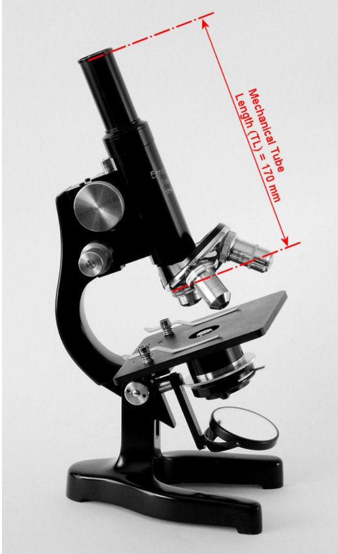
Figure 24 – Shows mechanical tube length of 170 mm for a Leitz LL student microscope.
