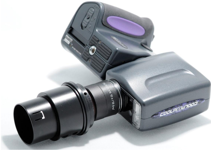
Figure 17 – Nikon Coolpix 990 with Periplan 10× ocular and custom adapter for the 38mm ISO port of the FSA binocular photo tube.
