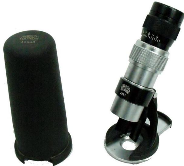
**Figure 4. Hensoldt “Tami” inspection microscope**
