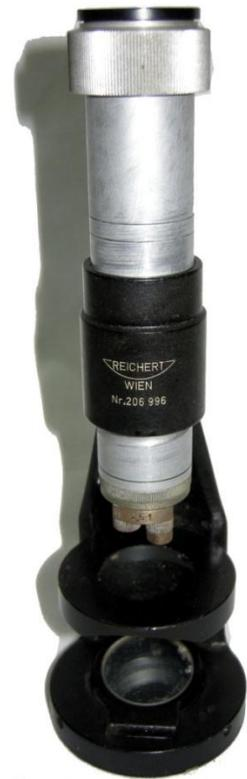
Figure 5. Reichert pocket microscope
