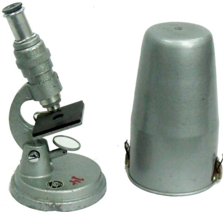
Figure 8. C&D Hemel Hempstead field microscope
