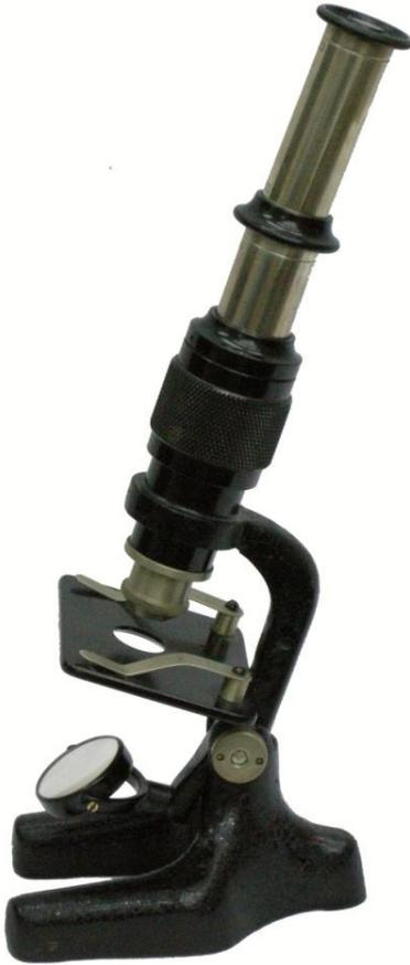
This is a version of the Tami but with a well-made solid cast iron stand. The draw-tube is marked with the magnifications, which are similar to those of the original Tami but are less detailed. The knurled helical screw focusing is also identical to that of the Tami. The optical quality seems to be lower than that of the original German microscope, but it is still useable.
