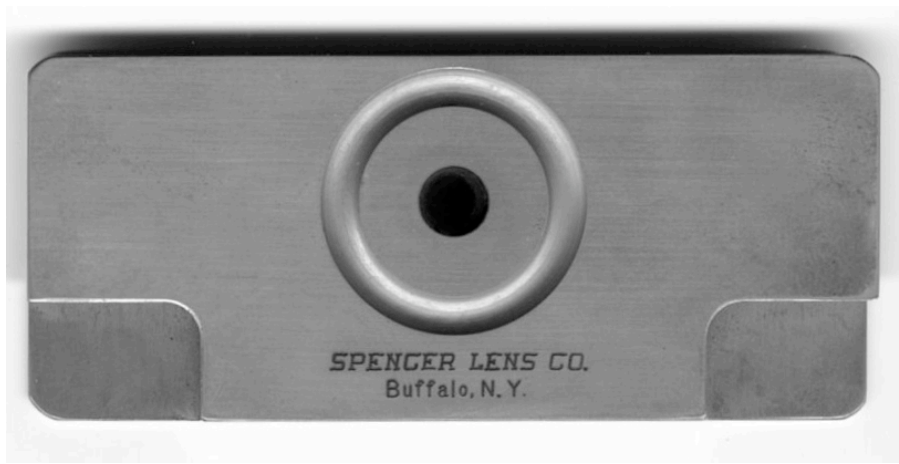
Figure 6. The upper surface of a Spencer on-stage dark-field condenser. The black, central area is the glass surface that allows light to reach the specimen. It is surrounded by a flat metal surface, and then by a groove that collects any overflow of immersion oil. Here, an optical illusion makes this groove to appear as a risen circle.
