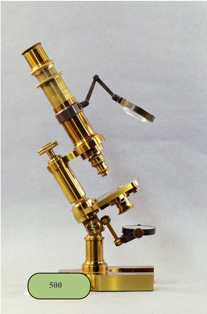
Figure 3 [#500]. A stand signed E(dmund) Hartnack & A. Prazmowski, Rue Bonaparte 1, Paris. The serial number 12460 indicates a circa 1880 date of manufacture. This is an elegant example of the “Continental” style microscope. This design inspired many European and American microscope makers for almost seven decades.
