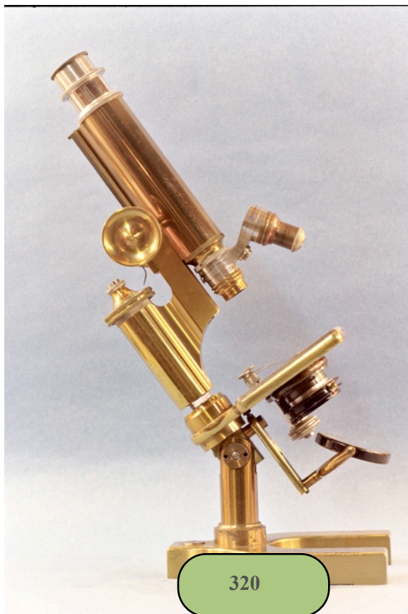
Figure 1 [#320]. A monocular "Continental style" brass microscope, Bausch & Lomb model BB4, serial #19609, from the late 1890s. Notice the unusually long working distance provided by the 48 mm low power objective.
