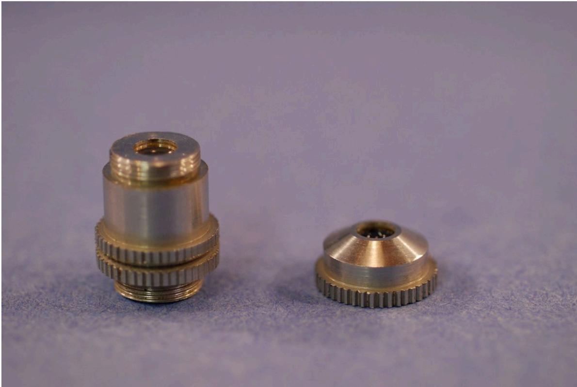
**Figure 3. The two components of the divisible objective; the one to the left attaches to the microscope body.**
