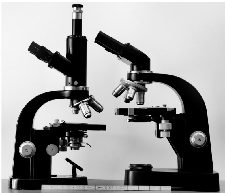
Figure 8: Side-by-side comparison between SM-D (left side) and Labolux-D (right side). The scale bar is in inch. Please note that both microscopes have the same focusing knobs.
