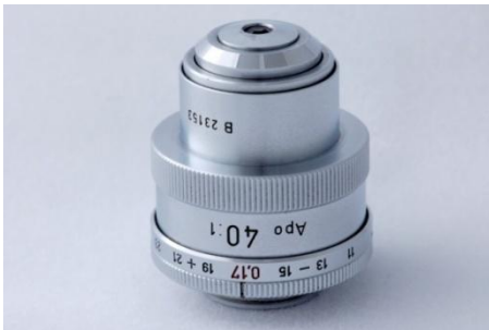
Figure 13: Leitz APO 40x NA 0.95 objective with correction collar. This is one of the many Leitz objectives produced during this time period.
