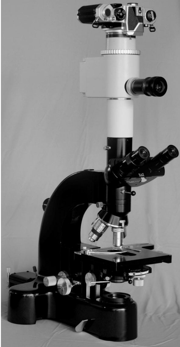
Figure 20: Leitz Ortholux with Nikon AFX camera system and Nikon FM SLR camera. For this picture, a Nikon FM is used instead of a DSLR. An Olympus NFK 2.5x photo eyepiece is used. It is added with a custom adapter in such a way as to capture the intermediary image produced by the objective.
