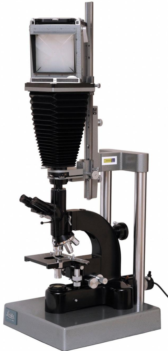
Figure 11: Leitz Ortholux with Leitz Aristophot. A 4x5" bellows -- camera is mounted to the Aristophot. A sleeve has been inserted into the light port for episcopic illumination.
