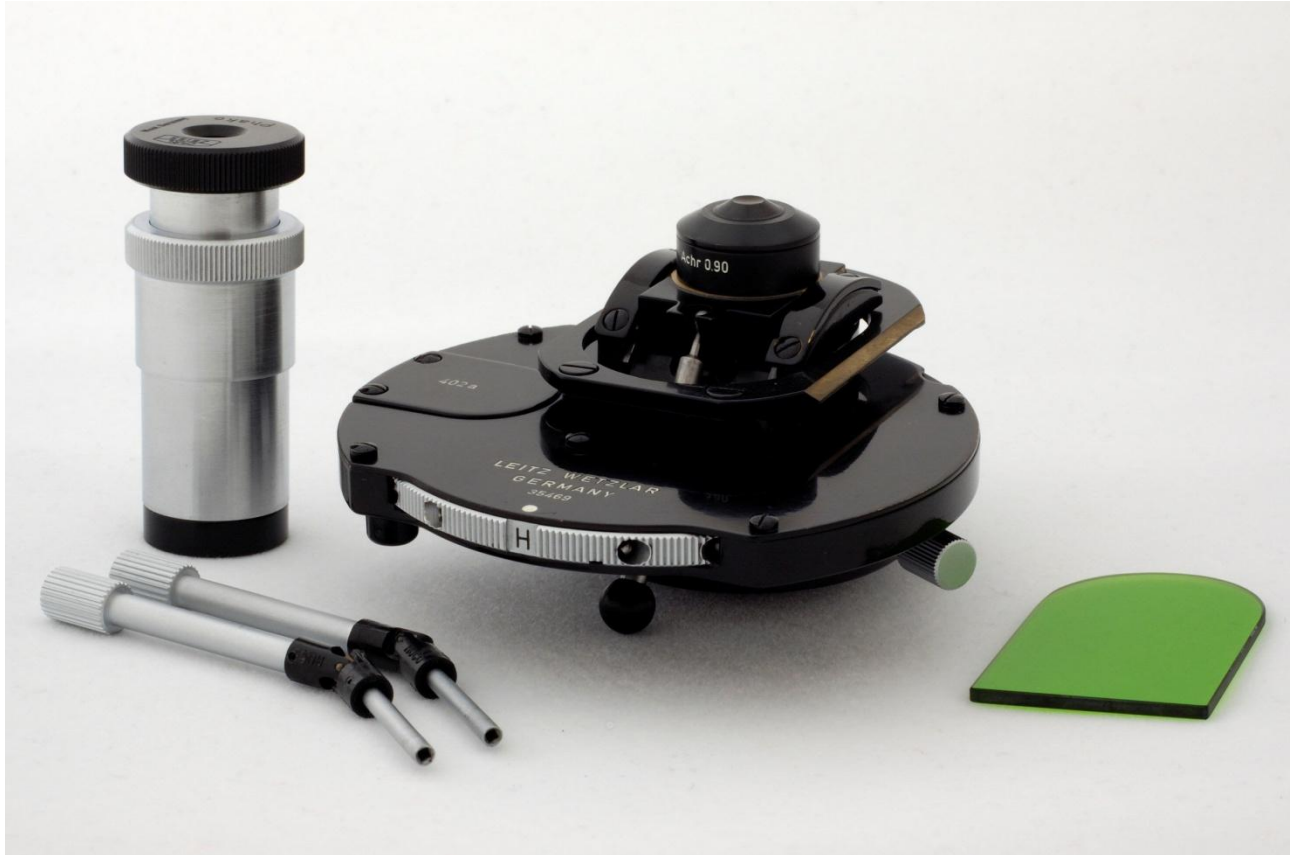
Figure 16: Leitz phase contrast condenser 402a with centering screws, green filter and phase centering telescope.
