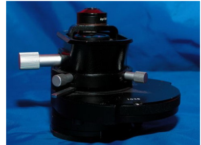
Nomarski DIC Condenser with Wollaston prisms, rotatable film polarizer at bottom; 1.25 aplanatic top lens
