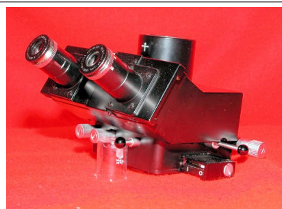
The two silver knobs on left of the black knob are for centeration of the Bertrand lens. The black knob controls the pin-hole stop.
