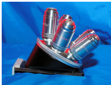
Standard 1X quintuple nosepiece with NPL Phaco lenses.
