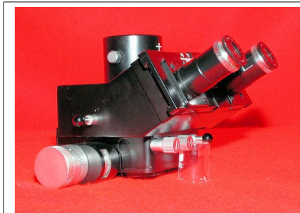
Left side view of FSA-50 body tube. The large silver knob on the bottom is the analyzer control drum that can be rotated 360° with an accuracy of 0.1°.
