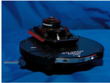
Phase contrast condenser 402A with 0.90 NA top lens
