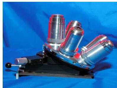
Centerable pol nosepiece with two filter slots, swing-in auxilliary lens for conoscopic image of small object detail.
