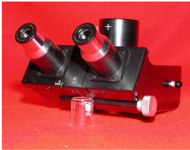
This is an FSA-55; the knob on the right controls the light either 100% to eyepiece or 100% to the trinocular tube. (The 10ml beaker is for photo positioning only!)
