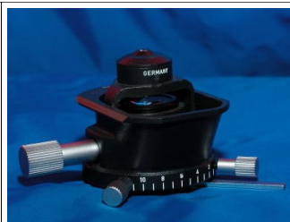
Condenser with detachable filter holder; 0.90 NA top lens
