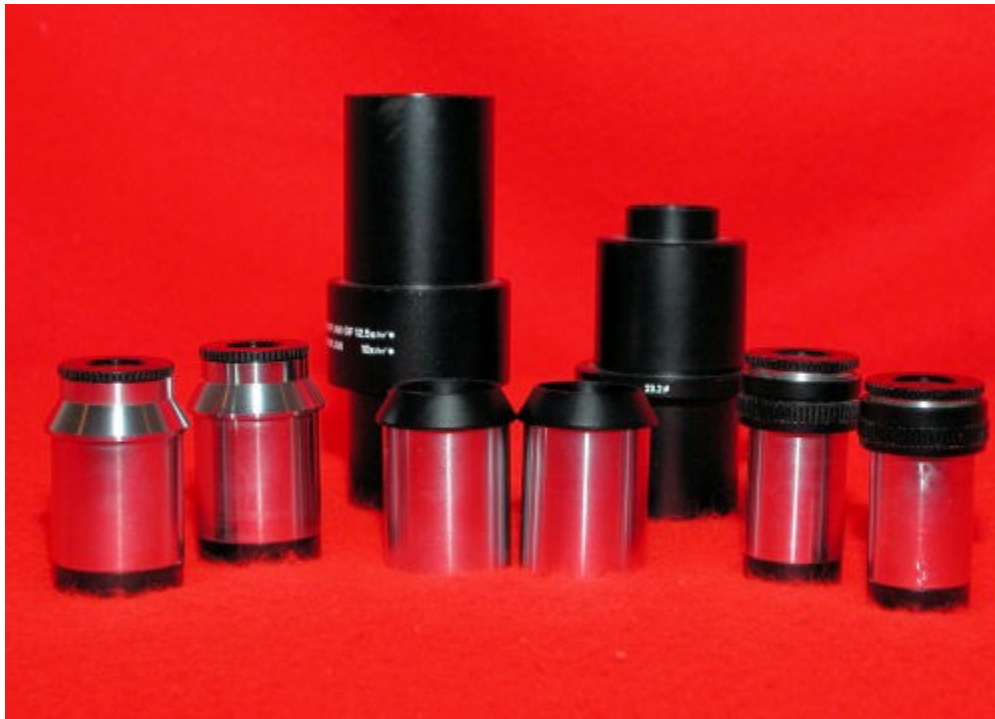
A comparison of GW (30mm) eyepieces on the left versus GF (23.2mm) eyepieces on the right. At the back are two photo tubes for use in the trinocular part of the body tube; center are adapter sleeves that allow the GF (23.3mm) eyepieces to be used in the FSA body tube.
