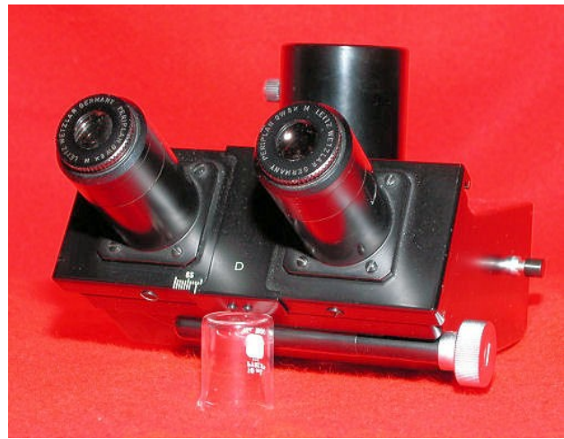
An FSA, the only difference between it and the FSA-55 is this model provided choice of 100% to eyepieces or 80% to trinocular and 20% to the eyepieces.
