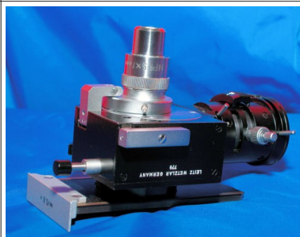
Pol vertical illuminator infinity corrected optical system, plane glass plate and compensating prism and auxilliary lens
