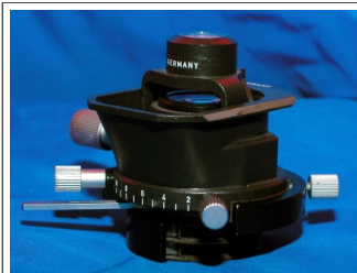
Condenser with detachable filter holder; 0.60 NA top lens.
