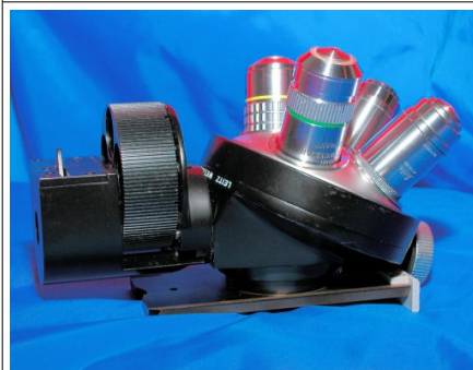
Epi-fluorescence after Ploem nosepiece. This uses standard 170 TL objectives.
